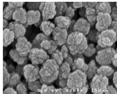
Fig. 4 SEM of colloidal silicalite-1 particles.
